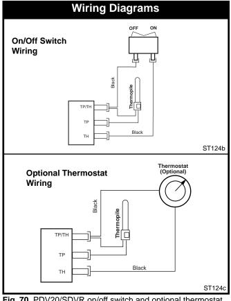
**Fig. 70** PDV20/SDVR on/off switch and optional thermostat circuit.
